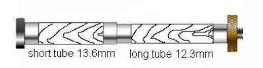
Turn outside diameter of the pen blank down to 13.6mm for the short tube, and 12.3mm for the long tube.
